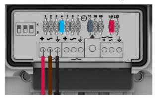
Blue Jumper - Sensor Position 4 Grey Jumper - Over run 10 Seconds Red Jumper - Pipe inlet 15mm
