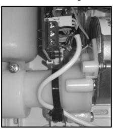
Before replacing the cover plate, ensure the cable runs in the recess groove:
