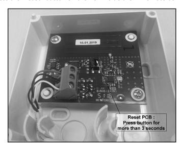
• Switch of the power to the pump circuit. Replace the lid to the RF remote box.
