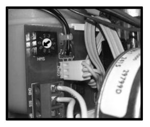
Tighten the cable tie and cut off the excess length:
