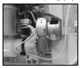
Before replacing the cover plate, ensure the cable runs in the recess groove:
