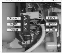
Wire connections to AKW Digital Pump:
