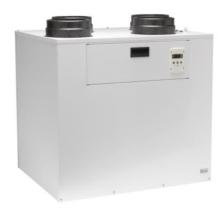
Ideal for 4 to 5 bedroom properties, the Natural Air 350 Mechanical Ventilation with Heat Recovery (MVHR) unit provides whole-house ventilation - supplying and extracting air through the entire property. Fresh air is supplied from outside the premises, while warm, stale, damp air is continuously extracted out.
