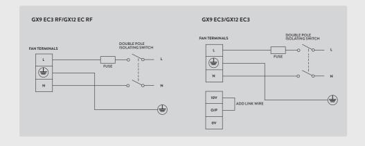
$\begin{tabular}{ll} \textbf{ANCILLARIES} \\ \textbf{We recommend the GX9 EC3 and GX12 EC3 RF controllers to operate the fans wirelessly.} \\ \end{tabular}$
