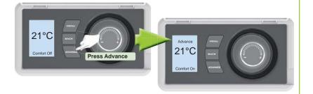
heater is in 'Comfort On' mode and you don't want heat, press the **Advance** button. The heater's change mode will go off until the beginning of the next 'Comfort' period, then go back to the timed heating periods.
