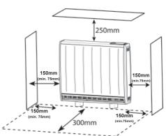
Do not place objects within 300mm of the front of the heater and 150mm (min. 75mm) either side.
