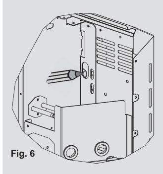
7. Six fixing positions must be selected for each model. Mark the positions for the fixing holes.Remove the bracket from the wall, drill the holes and fit the wall fixings best suited to the application.
