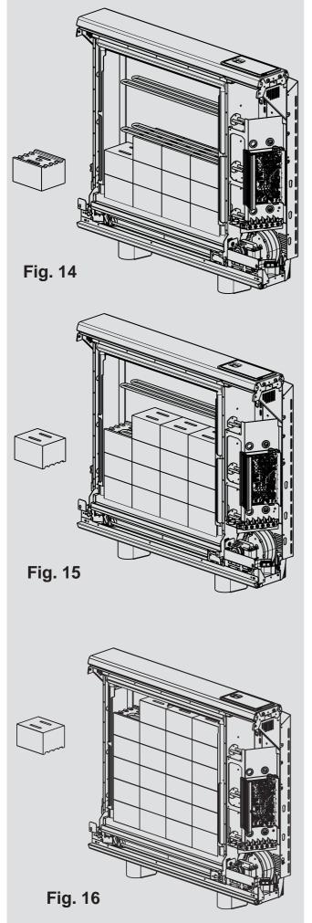
14. The third row of brick is positioned in a manner similar to the first row. Again be careful not to damage or dislodge the element.
