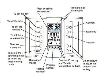
Percentage (%) of energy sent to the heating system to maintain the desired temperature.
