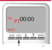
Once the P1 ON time is set, press **ENTER** and set the **P1 OFF** time (i.e. the time at which the heater should switch off).
