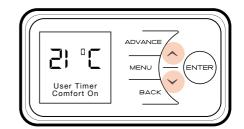
If you require a different room temperature use the **Up and Down** buttons until the display shows the temperature you require.
