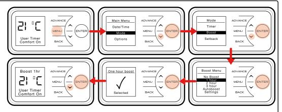
weather. You can select how long the boost will run for, from one to three hours. Once the boost has run for the selected time it will automatically switch off.
