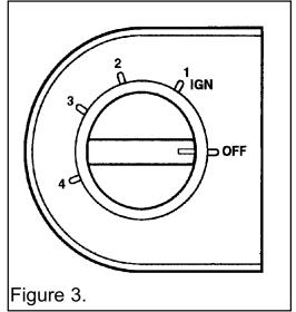
•The control knob should be depressed slightly before turning whenever you are changing the burner setting.
