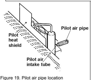
tube locates fully into the pilot air pipe attached to the back panel (See figure
