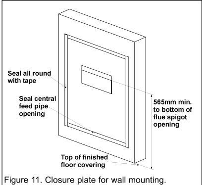
lighted match or smoke match to the flue spigot opening in the closure plate and observe the smoke. If there is a definite flow, continue with the installation. If not, check the fitting of the closure plate. The fireplace flue pull check described in section 6.3 should have confirmed that the fireplace itself is satisfactory.
