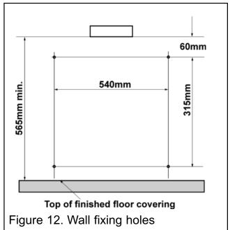
placing the fire in position and marking the wall through the holes in the back panel. Drill and plug the holes using no.10 wall plugs. Place the fire in position and secure with four no.10 x 2in. woodscrews.
