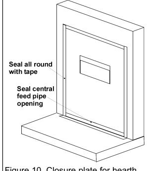
Figure 10. Closure plate for hearth mounting.
