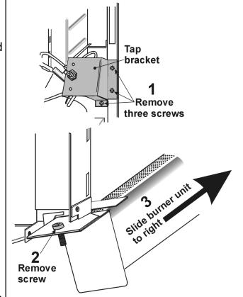
Figure 18. Burner module removal
