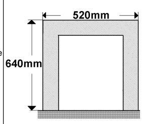
Figure 1. Area to be free of combustible cladding
