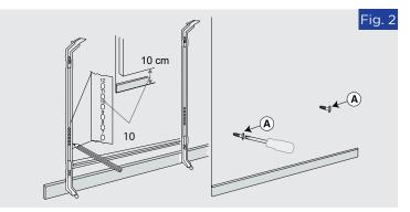
STEP 2: screws (A-A). Then fasten the wall bracket with the top screws. Place the heater on the wall bracket (1) and click the heater onto the top catches (2).
