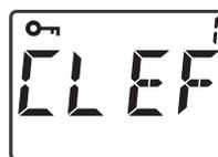
Press the + and – keys simultaneously for 3 s until **CLEF 1** and the symbol
