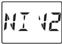
Press the and keys for 3 s until **NIV2** is displayed. Press the key for 3 s until the first parameter is displayed. Press the key to move onto the next parameter and, at the end, to return to manual operation.
