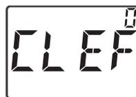
Press the + and – keys simultaneously for 3 s until **CLEF 0** is displayed and the symbol
