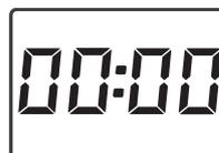
In this display, use the + and - keys to enter the time using the HH:MM format and then confirm by pressing . Each value can be changed when it flashes.
