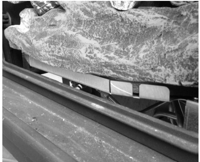
Figure 2b. Front log location on burner module
