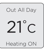
When the heater is trying to achieve or maintain a room temperature, 'Heating On' will be displayed, otherwise, 'Heating Off' will be displayed, during Timer modes only.
