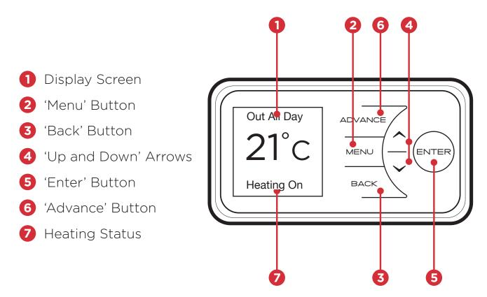
The heater is fitted with an adjustable thermostat enabling the room temperature to be controlled. The minimum room temperature is 7°C. The maximum temperature is set to 30°C. A temperature of 21°C is a common comfortable room temperature.
