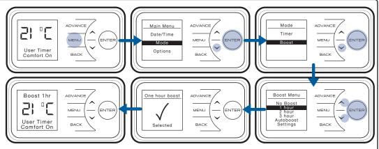
weather. You can select how long the boost will run for, from one to three hours. Once the boost has run for the selected time it will automatically switch off.
