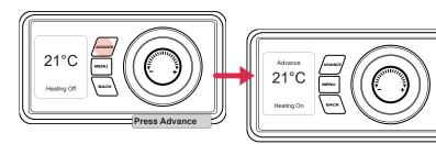
heater is in 'Heating On' mode and you don't want heat, press the Advance button. The heater's change mode will go off until the beginning of the next 'Heating' period, then go back to the timed heating periods.
