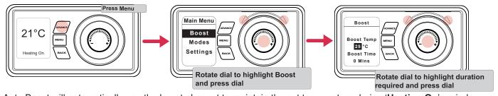
Auto Boost will automatically use the boost element to maintain the set temperature during 'Heating On' periods. Note: Boost element uses peak rate electricity and could lead to increased running costs.
