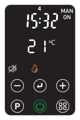
• In the event of a power interrupt, plugged out/power cut/tilt switch operation, then reconnected the appliance will return in Standby mode, once turned back on the product will return to last used settings.
