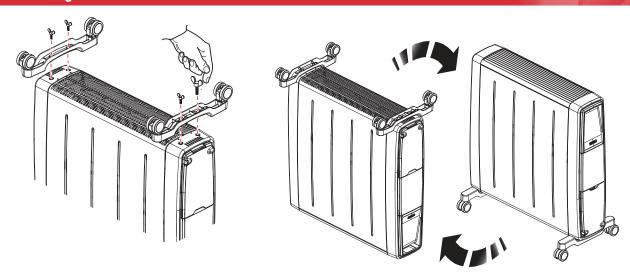
WARNING: The radiator must only be operated with the wheels and castors securely fitted and in the upright position.
