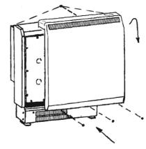
Take care not to trap wires or the thermostat capillary between the panel flanges. Ensure all washers are replaced in their original positions.
