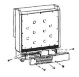
The top panel and front panel are joined and should be removed as one assembly. To do this, remove the screws fixing the rear flange of the top panel, and remove the screws along the bottom edge of the front panel. Carefully swing out bottom of front panel and lift assembly clear of casing, this operation also removes the control knobs under the flap. Put assembly in a safe place to avoid damage to
