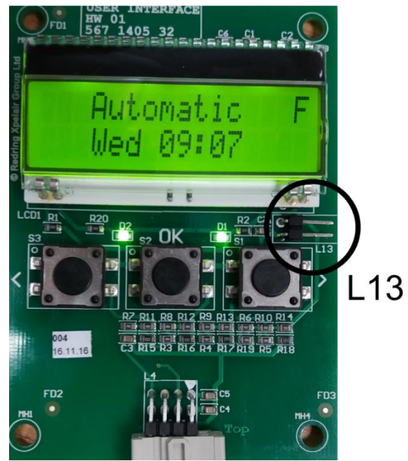
Fig. 6.12B Display circuit board without jumper L13
