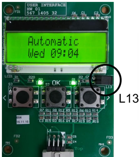
Fig. 6.12A Display circuit board with jumper L13
